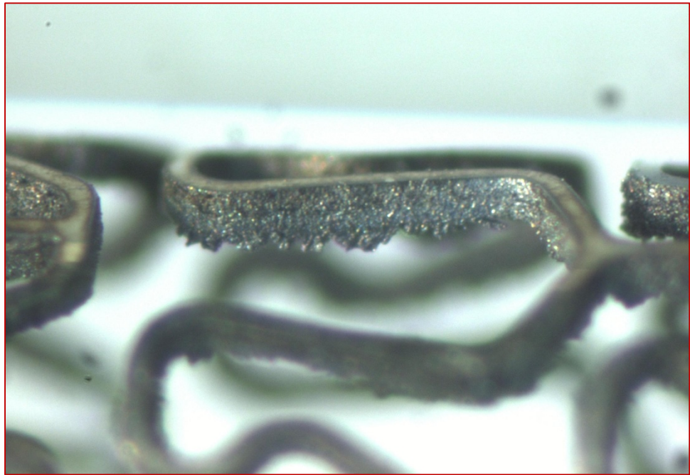
Figure 3: The vascular stent above was machined with a nanosecond laser. It exhibits thermal damage in the form of burrs and other heat affected zones (HAZ). A part like this would require several re-work steps, including manual honing and chemical etch steps to clean up the thermal damage.
